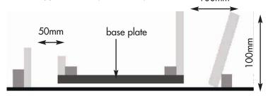
Cross-section of typical grouting formwork
